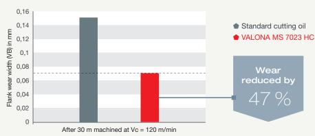
VALONA MS 7023 HC decreases wear while improving surface quality and edge resistance when machining stainless steels.
