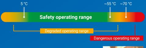
In case of cell failure, a thermal runaway can occur, causing an important emission of gases and a possible fire.
