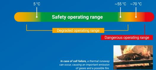
The optimized cell operating temperatures guarantee long-term battery capacity and performances.
